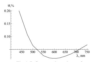
Fig. 1. Reflectance dependence of a substrate covered with nano-particles layer on the wavelength of incident light.
