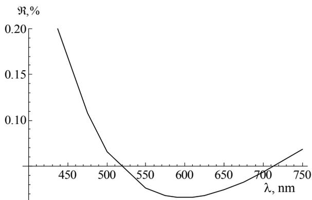
**Fig. 1. Reflectance dependence of a substrate covered with nano-particles layer on the wavelength of incident light.**
